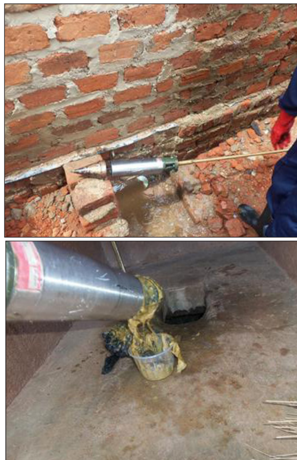
Figure 3 Pit sludge sampler (Makerere University, 2015)
