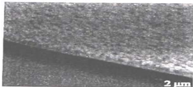
Fig. 8. SEM images much closer view for thickness of the beam measurement
