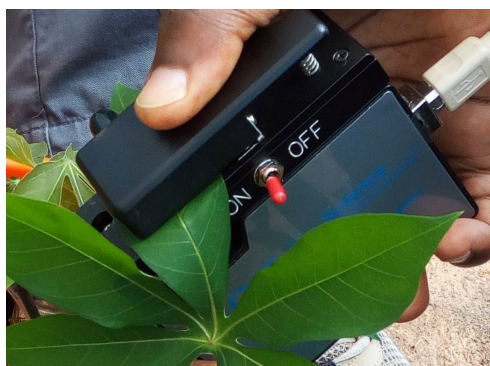
Figure 1: Data collection with a CI-710 miniature leaf spectrometer [4].
