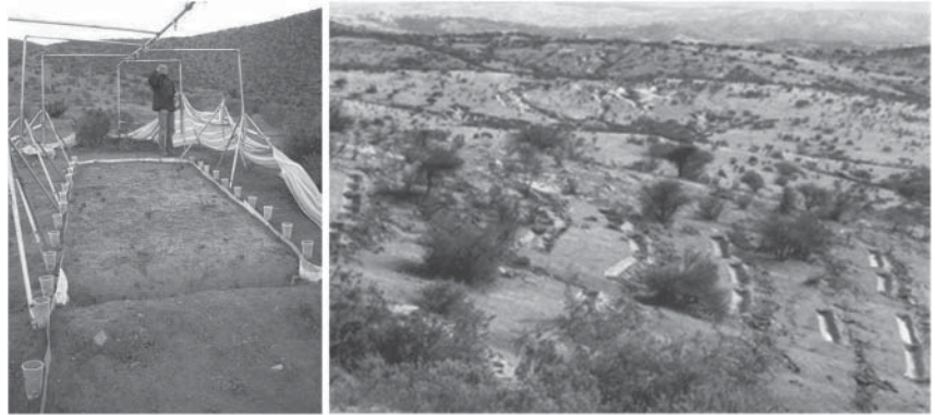
Figure 4.1 Hillslope with impluvium, infiltration trench, and 10 m-long rainfall simulator in the Elqui Valley, Chile (left), and watersheds with (front) and without (back) infiltration trenches in the Metropolitan Region, Chile (right).
