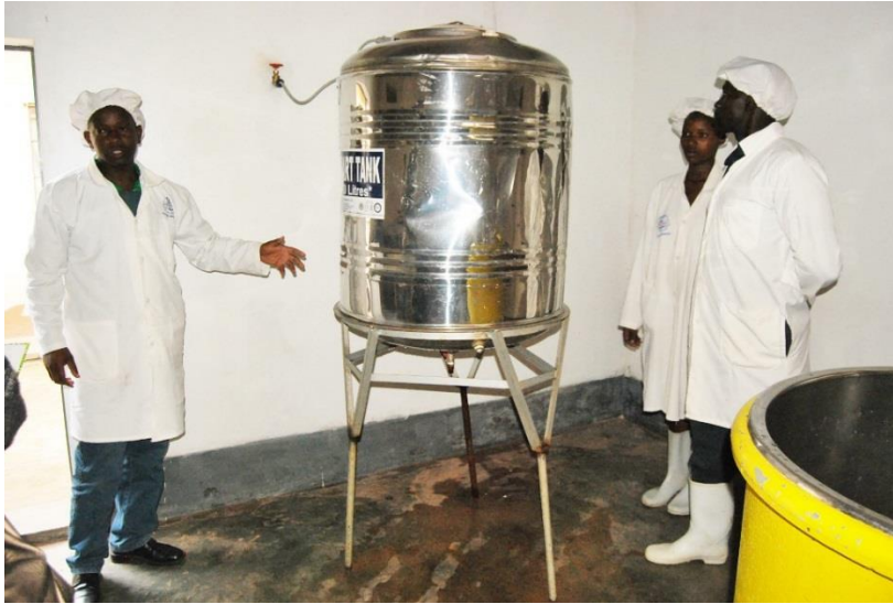
Figure 5. Water treatment system (450lt capacity)
