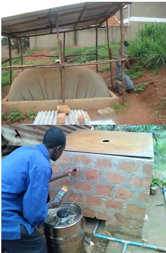
Fig. 2. Researchers perform a cooler regeneration experiment using biogas produced by a “bubble” digester fed by 5 zero-grazed cows. The cooler is the stainless steel vessel with a black cap the mild steel plate on top of the regenerator is removed and the cooler placed inside the double walled brick structure. The cooler is heated from the bottom through a burner. During regeneration, a layer of bricks is placed on top of the mild steel plate for insulation purposes. The ratio of the mild steel plate exhaust hole to the air inlet opening in front of the regenerator is a key design parameter in achieving a desirable temperature inside the regenerator.
