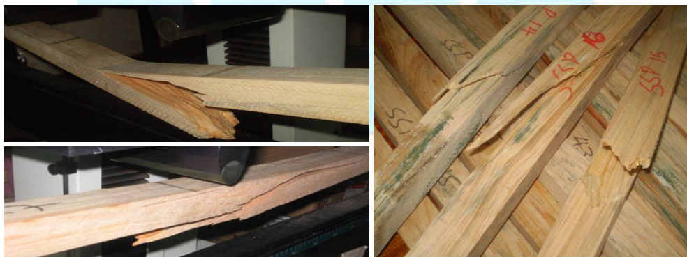
Figure 8: Failure Modes during Structural Size bending test – P. Caribaea
