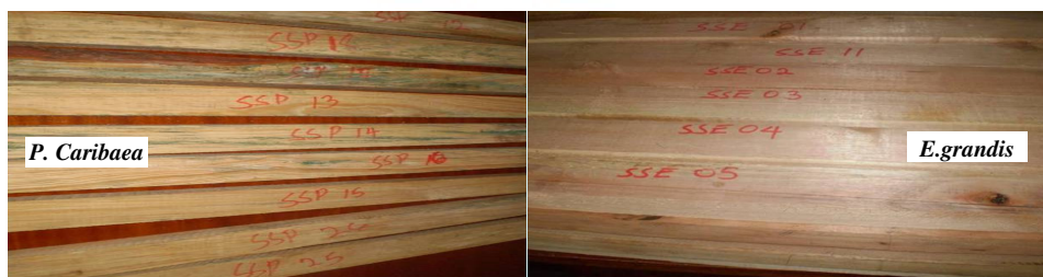
Figure 1: Structural size specimens for Eucalyptus grandis and Pinus caribaea
