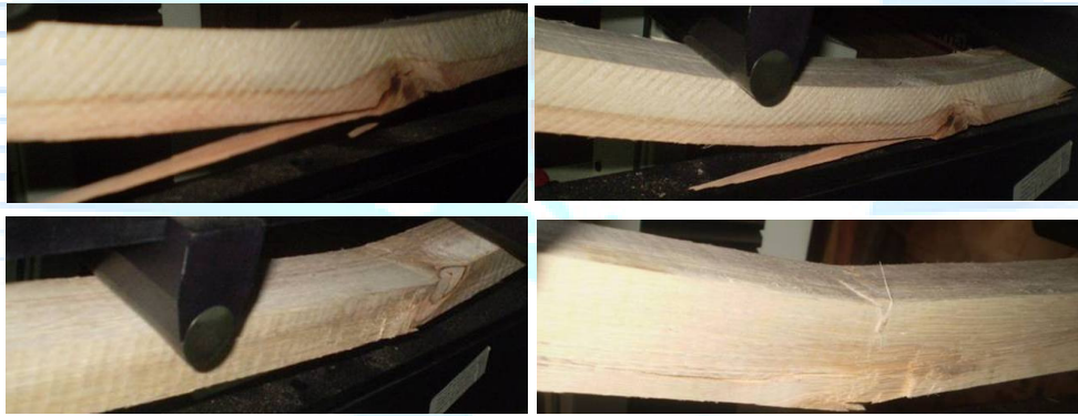
Figure 7: Failure Modes during Structural Size bending test – E. grandis
