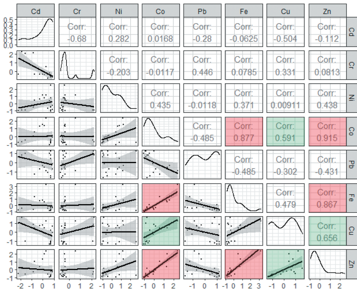
Figure 3. A generalized pairs plot displaying paired combinations of standardized levels of Cd, Cr, Ni, Co, Pb, Fe, Cu and Zn in cabbage, dodo , scarlet eggplant and tomato samples collected from open markets in Bushenyi, Ishaka, Kashenyi, Kizinda and Nyakabirizi (Bushenyi District, Uganda). Strong and positive correlation between Fe and Co, Zn and Co, and between Zn and Fe are color coded red; moderately positive correlation between Zn and Cu, and between Cu and Co are color coded green.
