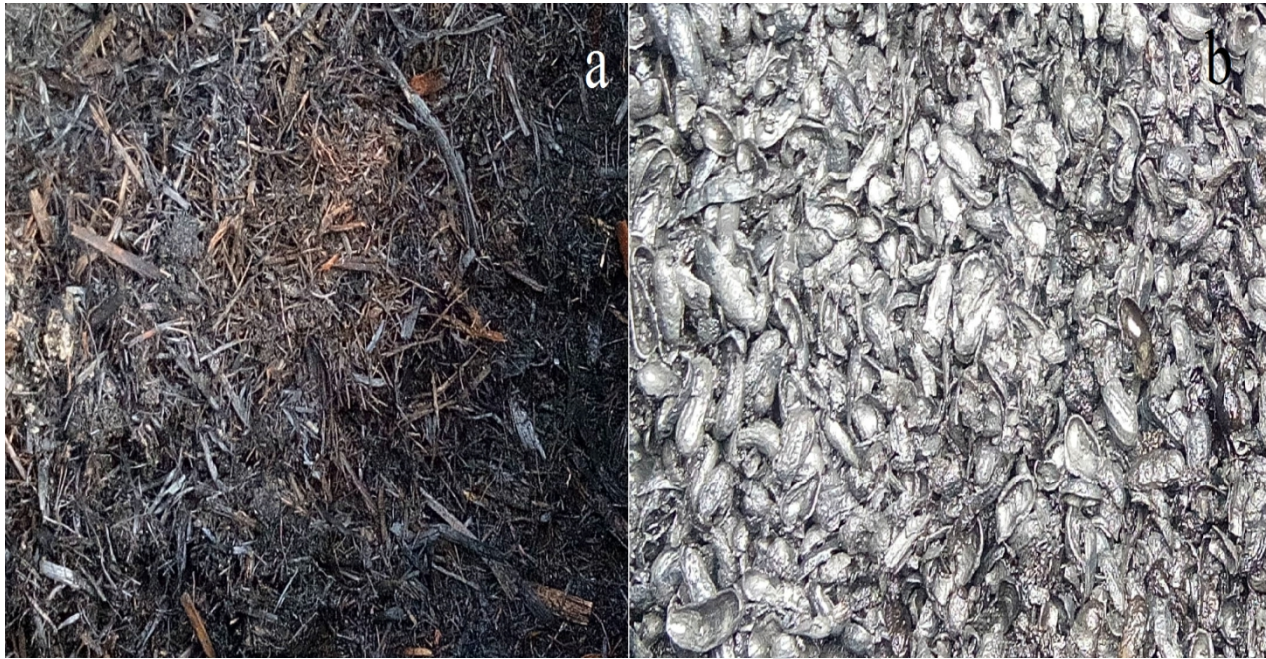
Figure 4: Picture of bio char of (a) bagasse, and (b) groundnut shells after carbonization
