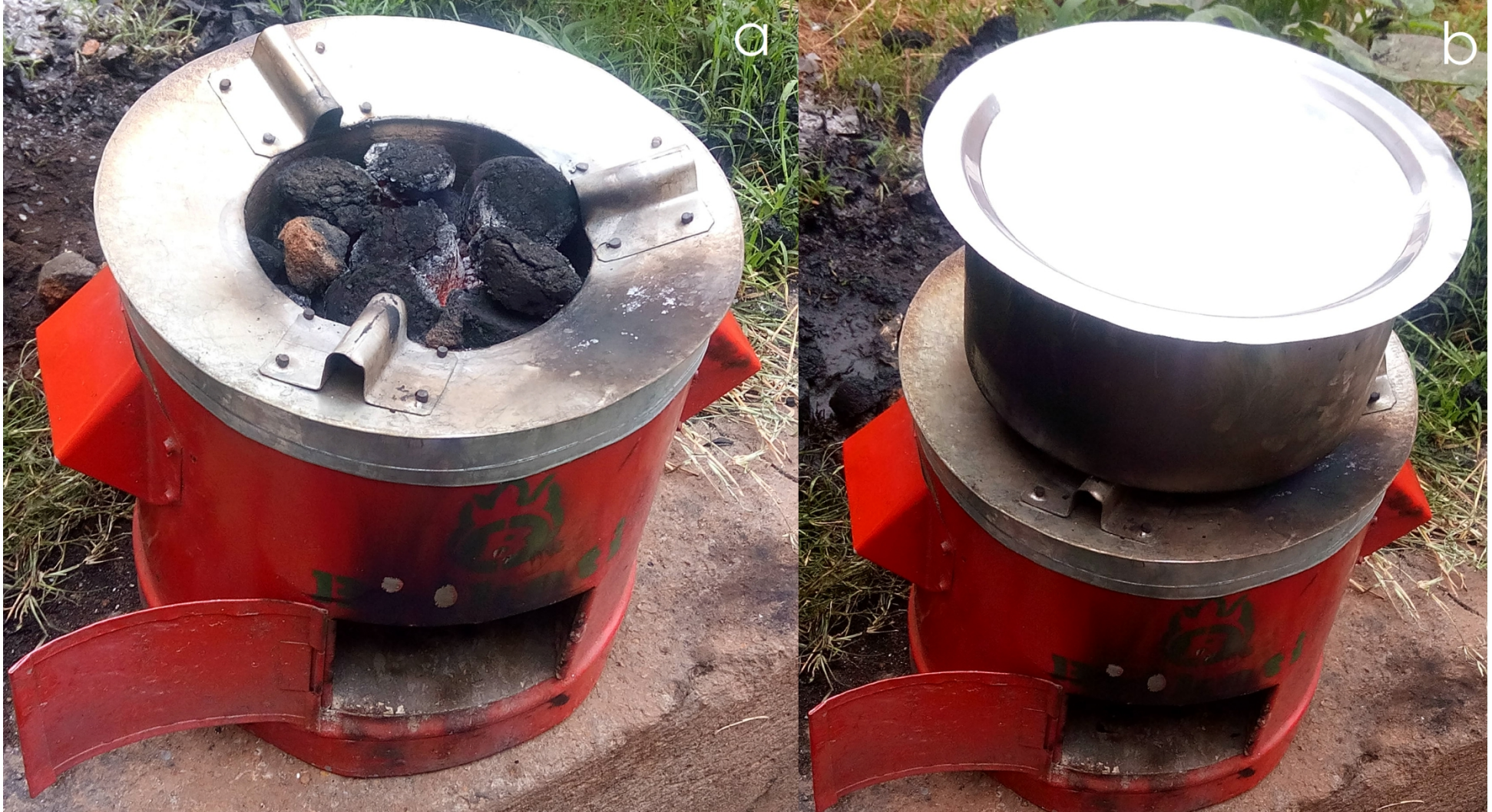
Figure 18: Improved cook stoves with ignited briquettes (200 g) (a) boiling 0.5 liters of water (b).
