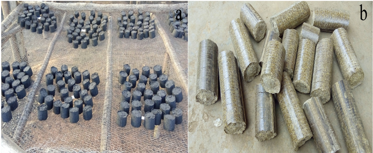
Figure 5: Picture of carbonized (low pressure) briquettes (a) and non-carbonized (high pressure) briquettes
