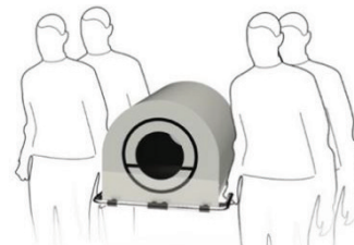
Fig. 8. The magnet, despite its weight (100 kg), can still be lifted by 4 persons.
