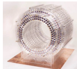
Fig. 2. The (permanent) magnet in Halbach arrays in which the patients are inserted [11].
