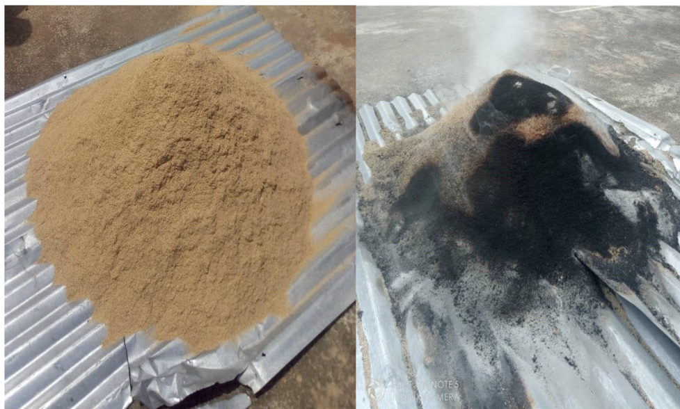
Fig. 8. Rice husk and ash processing by direct combustion.
