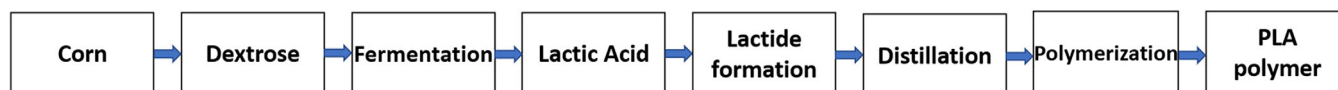
FIGURE 2 PLA's synthesis path (adapted from ref. [21] ) [Color figure can be viewed at wileyonlinelibrary.com]
