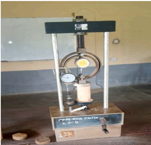
Fig. 3. Unconfined compressive strength experimental setup.
