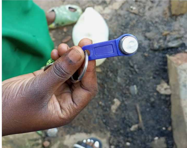
Figure 4 | Tokens, a key accessory to access safe water on PPDs. Author photos taken in Bwaise II, Kawempe Division.
