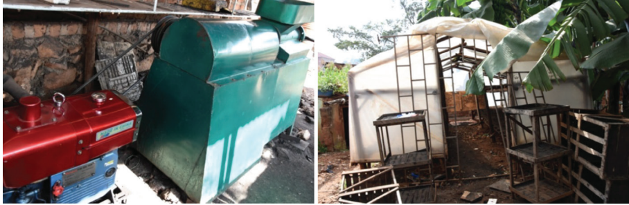
Figure 3: Image of briquette-making machine (left) and solar dryer in proximity of a small banana garden (right)
