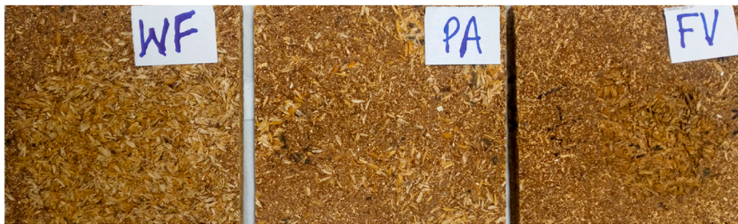
Fig. 2. Particleboards developed using sawdust, rice-husks and adhesives WF, PA, and FV.
