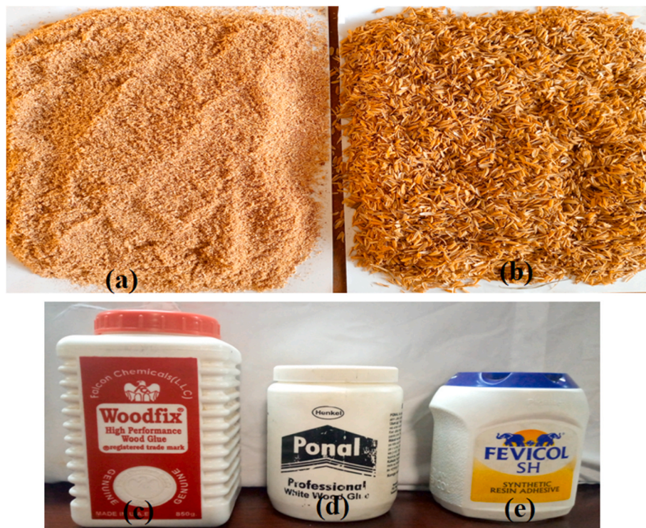
Fig. 1. Raw materials used (a) saw dust, (b) rice husks, and adhesives packs (c) Woodfix, (d) Ponal, (e) Fevicol.
