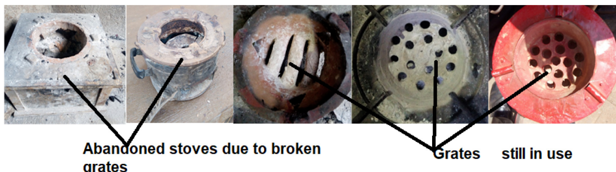
Fig. 1. Some of the charcoal cook stoves no longer in use due to damaged grates as compared to those with working grates.
