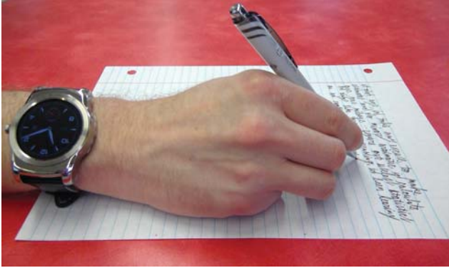
Figure 1: A user in the middle of writing a paragraph. As the fingers and pen meticulously trace out the strokes forming each character, the watch, largely constrained by the table-top, undergoes limited motion relative to the pen tip. We investigate the question of whether these subdued movements could capture the user-specific traits exhibited at the much more mobile pen tip.
