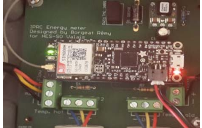
Fig.4. Adafruit Feather 32u4FONA with GSM module
