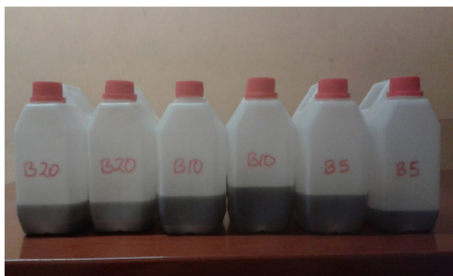
Fig. 3. Bio-oil/diesel emulsions three months after production.
