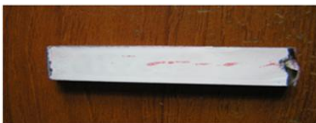
Fig.4: Centerline crack, PV5
