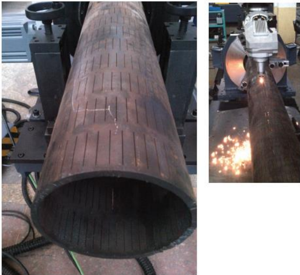
Fig. 5. A slotted steel pipe used in the oil industry for heavy oil production; the slots are created by laser cutting (Rath and Gaebler, 2017).
