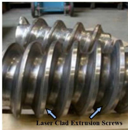
Fig. 7. Laser cladding of pet-food granulate extrusion screws extends screw lifetime (Laser Cladding Venture (LCV), 2017)
