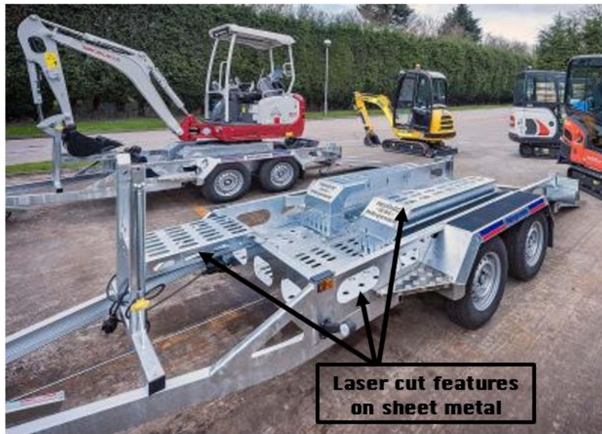
Fig. 3. Trailer body with sheet metal component parts having laser-cut holes and slots (Larcombe, 2017).
