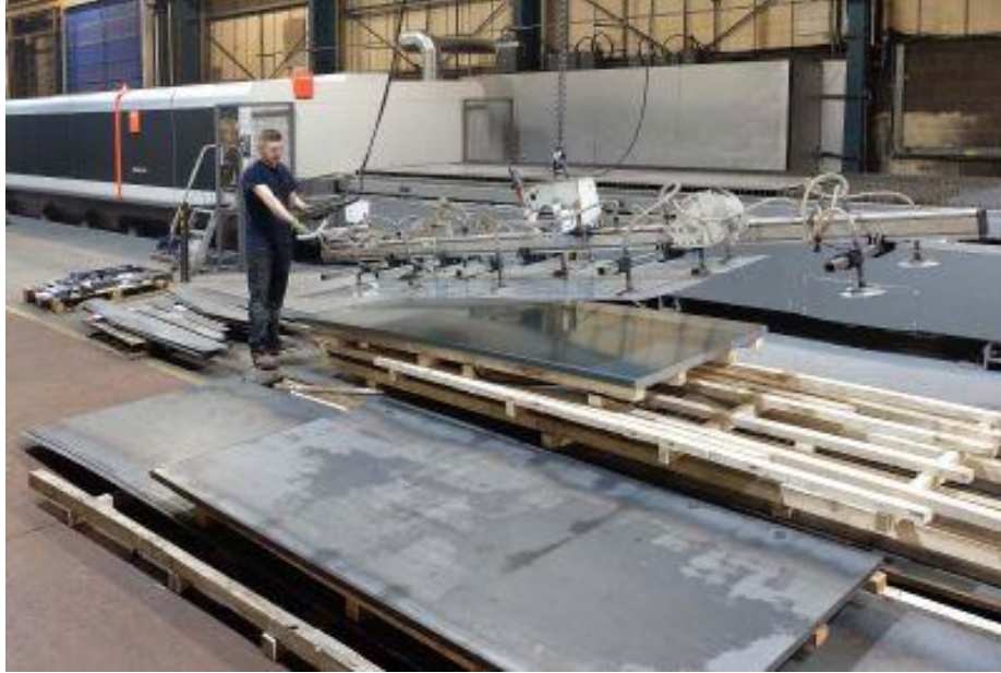
Fig. 4. A suction-pad lifting system for manually transferring sheet metal on and off the laser cutting shuttle table (Larcombe, 2017).
