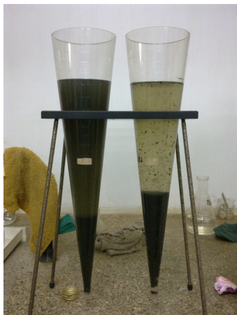
Figure 6: Conditioned lined pit latrine FS (left) and septic tank FS (right) at a dosage of 1 mL/gTS.
