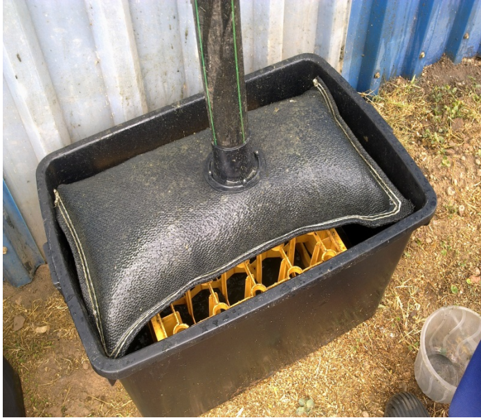
Figure 4: Geotextile pillow loaded with FS.
