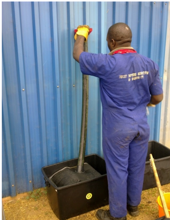
Figure 3: Loading of geotextile pillow with conditioned septic tank FS.
