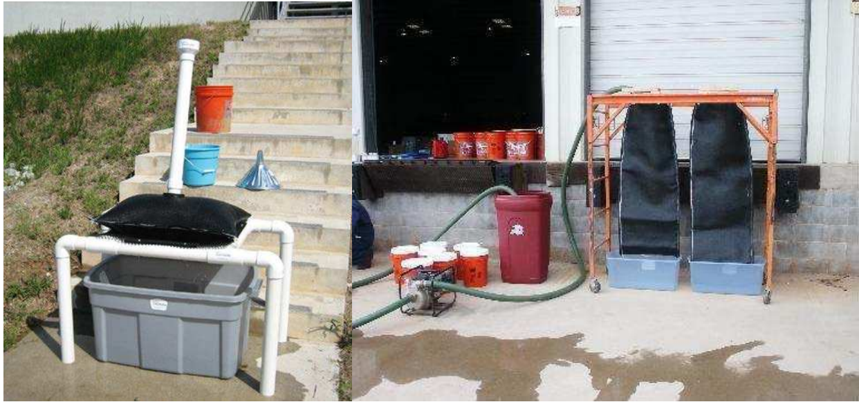
Figure 2: Experimental set up of GDT (Left) and HBT (right) (Tencate;2007)
