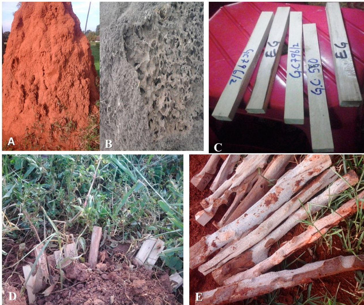
Figure 3. Eucalyptus wood damage following exposure to M. bellicosus and M. subhyalinus : (A) M. bellicosus mound, (B) M. subhyalinus mound, (C) wood stakes following exposure to termite damage, (D) wood stakes half inserted in the soil in proximity with termite mounds and mud tubes and (E) wood stakes after exposure to termite attack.
