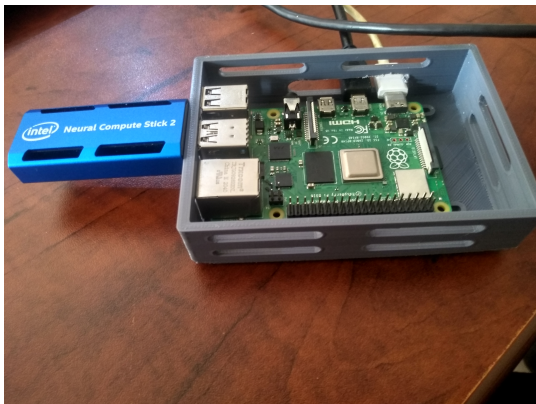
Figure 6: The 3D Packaged Edge Device System: A Raspberry Pi microcontroller and the Intel Neural Compute stick enclosed in a 3D printed casing.
