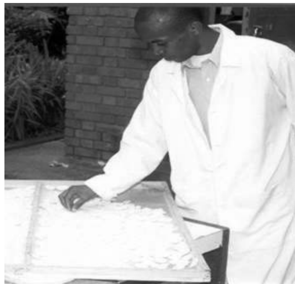
Figure 1 Spreading of banana slices on a tray before loading into the dryer.
