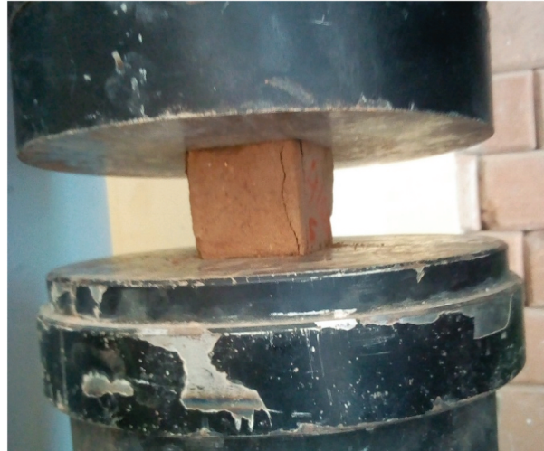
Figure 4. Failure pattern of the lateritic brick indicating delamination of the outer surface.
