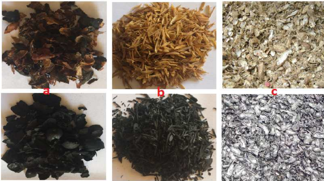
1 2 Figure 1: Agricultural residues before (Top) and after carbonization (bottom) to form bio-char: 3 coffee husks (a), rice husks (b) and groundnut shells (c). 4
