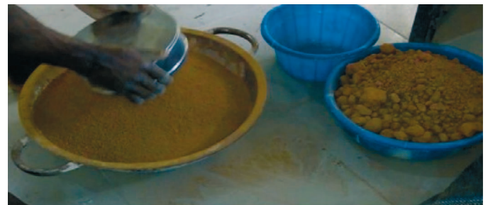
Figure 3. Reference soil preparation by sieving through a 2 mm aperture sieve.
