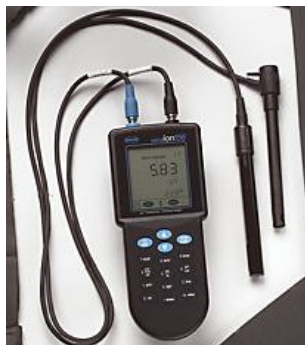
Figure 3. 2: Hach sensION156 portable multiparameter probe
