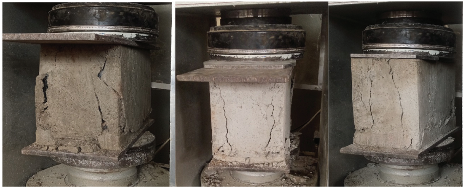
Figure 15. EBB block failure (left), PSB block failure (centre), SDB block failure (right).
