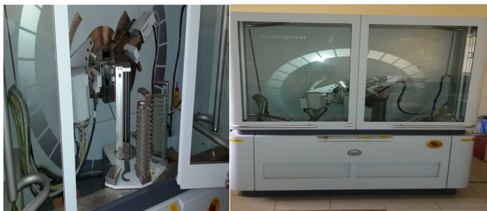
Fig. 4. X-Ray Diffractometer Experimental Set-up.
