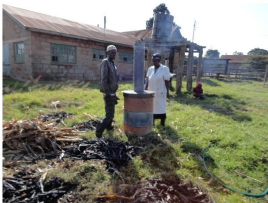
Photograph 21: Small-scale biochar making kiln at KARI Muguga South
