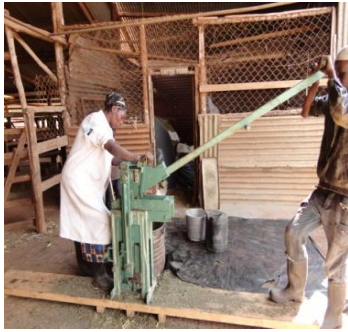
Moulding process Experimental feed blocks Photograph 22; Demonstrating use of biochar to mass produce feeding blocks
