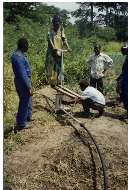
Photograph 17: On-farm evaluation of the treadle pump in Luwero
