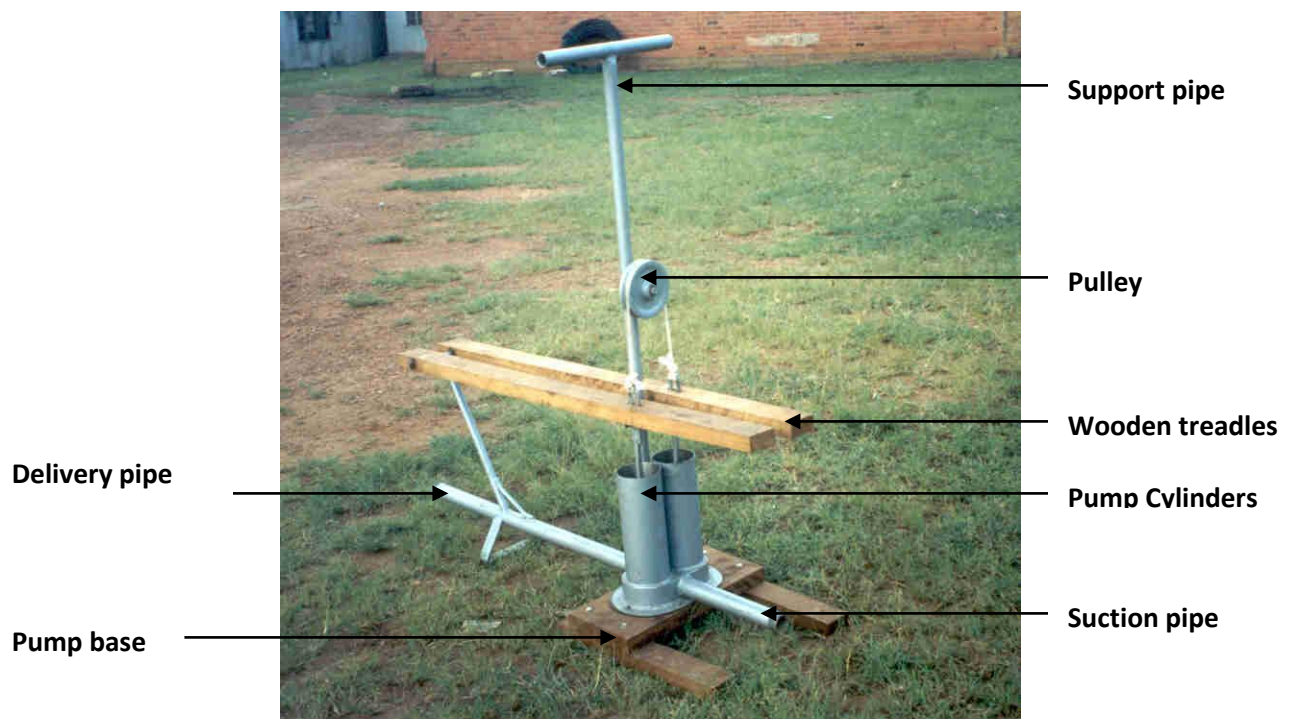
Photograph 16: Components of a treadle pump
