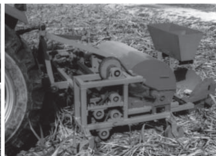
Fig. 5 IISR trash handling equipment
