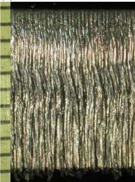
FIG. 10. Effect of cutting speed on dross attachment.
