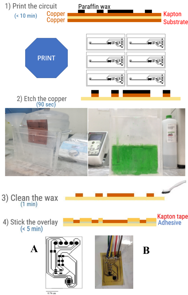
Fig. 4. Top: Printed Circuit Board Manufacturing Process. Bottom Left (A): Schematic for flexible printed circuit board. Bottom Right (B): Flexible IMU printed on film substrate with soldered wire touchpoints.
