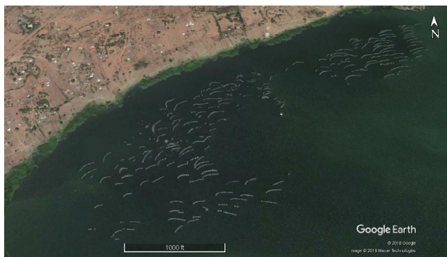
Fig. 3. Example of a cage aquaculture installation with a large number of cages (about 3140) on Lake Victoria, Kenya (Location coordinates (decimal degrees): Lat: -0.09581 ; Long: 34.07928 ).
