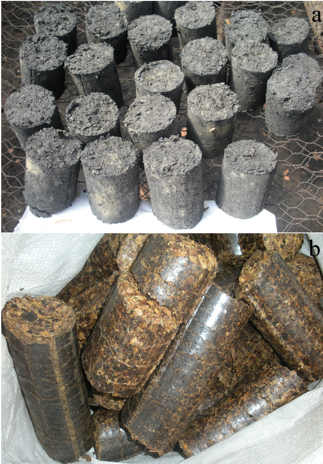
Figure 2: Samples of briquettes developed under low pressure after carbonization (a) and non-carbonized under high pressure development
