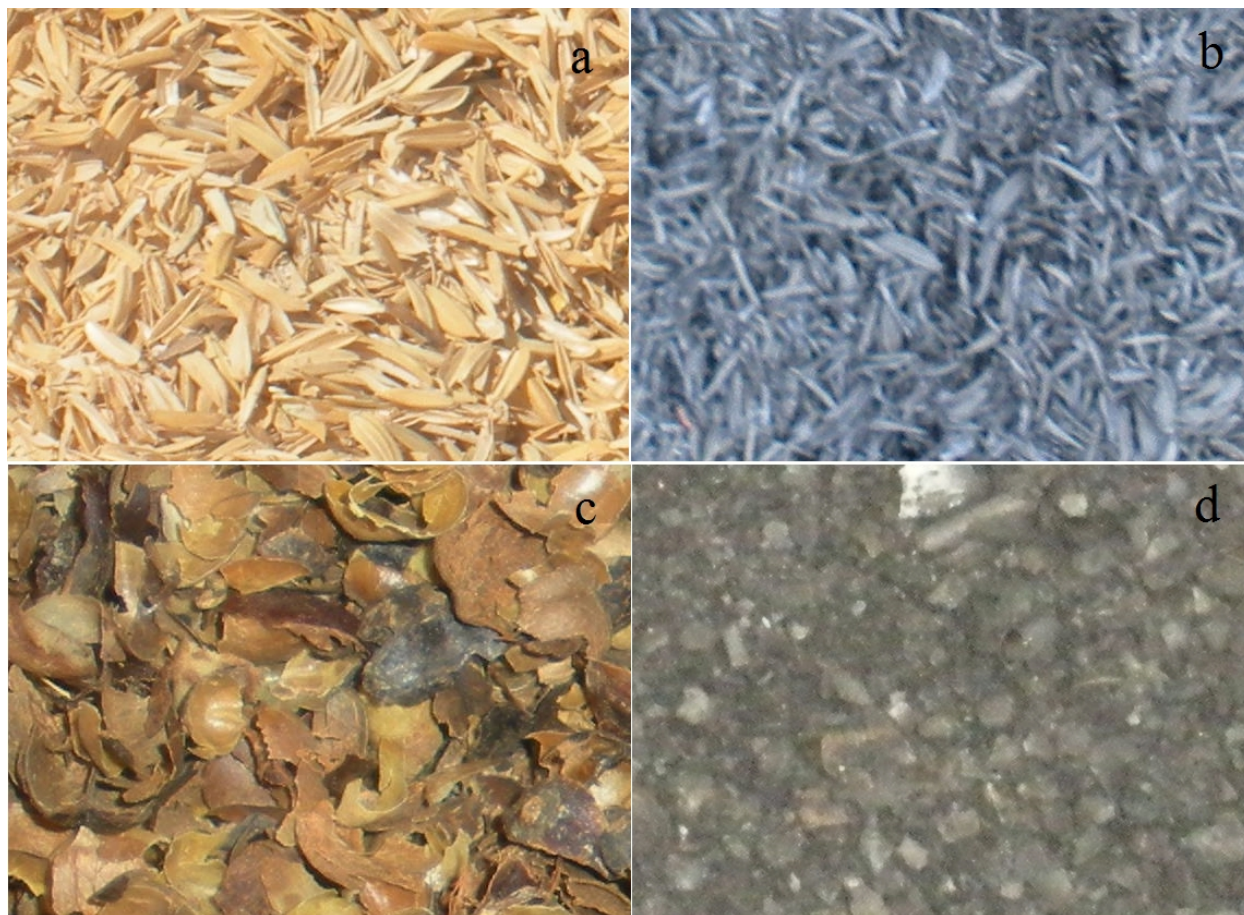
Figure 1: Picture of rice husk and coffee husk raw material, before (a and c) and after (c and d) carbonization
