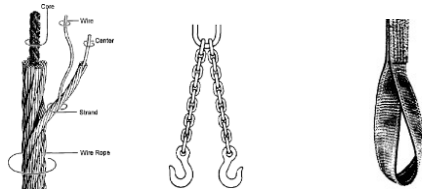
Figure 3: Rigging equipment - wire rope, chain sling, and synthetic web sling (Source: DOE, 2012).
