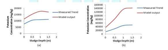
Figure 10: Measured and modeled concentration profiles for potassium in (a) lined pits and (b) unlined pits
