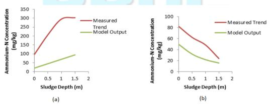
Figure 6: Measured and modeled concentration profiles for ammonium-N in (a) lined pits and (b) unlined pits
