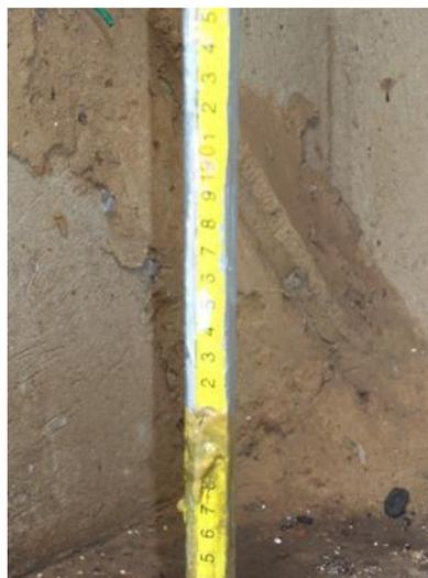
**Figure 3.** Depth tool with sludge markings.
