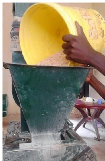
**Figure 1.** “Posho” mill grinding legumes to create flour.
